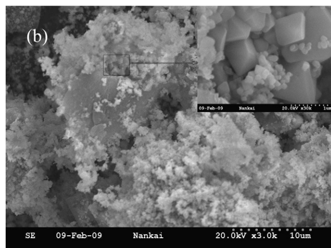
Fig. 4. SEM images of the products synthesized via hydrothermal reaction (a) and high temperature solid-state reaction (b). SEM images at high magnification are inserted.
